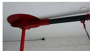
Twist handle until UPCLIMBER EXPAND is firmly tensioned between floor and ceiling
