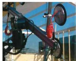
A two-circuit vacuum system ensures that the suction discs always have 400% overcapacity. A visual - and an acoustic alarm ensure that the machine is not operated until the system has reached optimum suction power. This makes the vacuum system one of the safest systems in the world.
